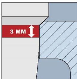
The first part of the stroke does not control any flow but is just energizing the different control stages. Moreover it is avoiding hammering during opening.
