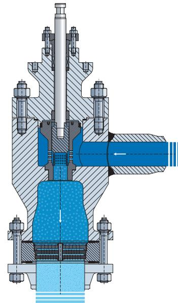
Throttling plates can be used to control the flow between the valve and the drain vessel.
