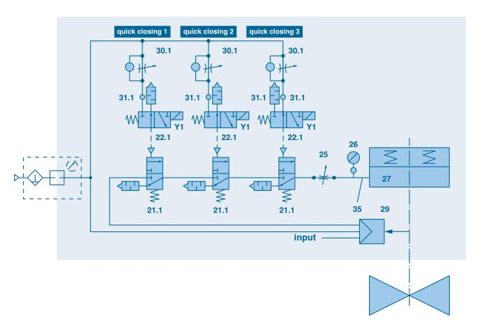
Schematic showing a quick closing device based on EN 12952-3 / TRD 421. The 3 quick pneumatic valves discharge the air from the "spring to close" pneumatic actuator and are also closing the air supply from the positioner when the quick closing valves are activated.
