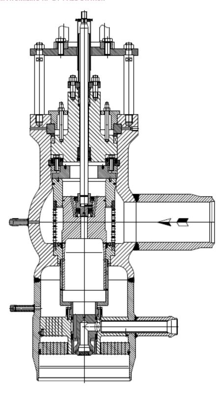
Ball shaped PRDS made of forged material equipped with a pressure seal, perforated cages with a pressure balancing system and an integrated steam atomizing unit
